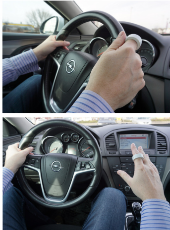
Figure 1. A smart ring enables tap-based input with the thumb while the hands are kept on the steering wheel (top image) and removes the need to move the hand and fingers to use controls placed on the steering wheel. The smart ring can also be used to articulate mid-air gesture commands (bottom image), removing the need for gesture acquisition sensors to be installed inside the vehicle. Note: for these photographs depicting illustrative use case scenarios for smart rings inside the vehicle, we used the Ring Zero device ( https://www.amazon.com/Ring-R001-PB01-ZERO-S-Black/dp/B00U8IX7DQ ).
