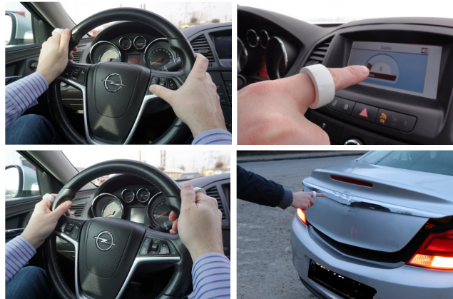
Figure 3. Top: combining smart rings with other input modalities inside the car: steering wheel controls and touch input. Bottom-left: using two rings for bimanual gestures. Bottom-right: interaction outside the vehicle.
