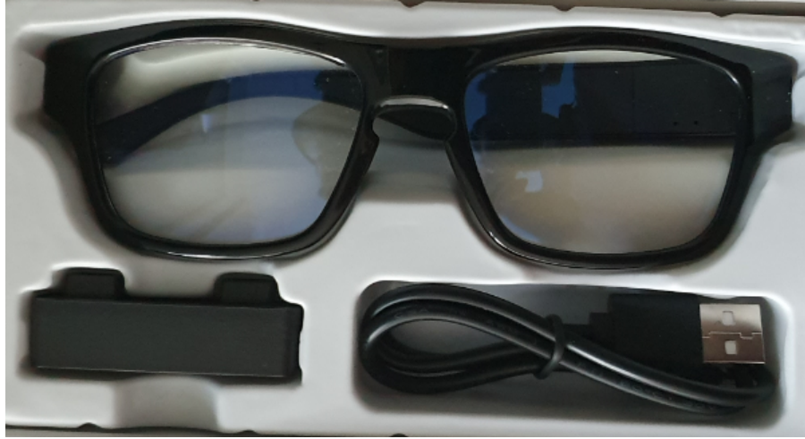
Fig. 2. The WI-G5 glasses [70] with a micro video camera embedded in the temple. Can you spot the camera? Advanced miniaturization at a low cost turns such devices into genuine threats for bystanders privacy, as reported in the studies from the literature [23,39,48], some conducted with considerably less inconspicuous devices.
