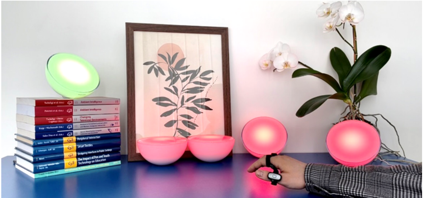
Figure 1: Tap4Light is an interaction technique based on finger tap gestures, designed to control smart lighting systems. In this photograph, five Philips Hue lamps are mapped to the five fingers of the hand, and are controlled, via the Tap Strap 2 wearable device, with tap gestures: a tap with one finger turns on, turns off, or selects the corresponding lamp, according to context; a tap with two fingers increases the brightness of the currently selected lamp; see Figure 2 for the entire gesture set.
