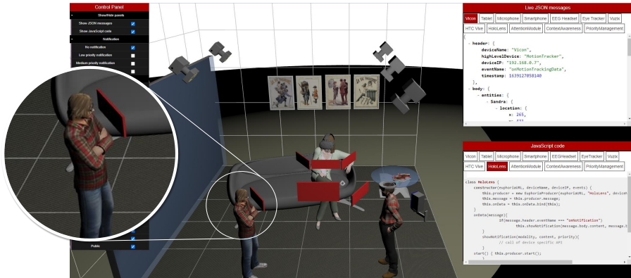
Fig. 1 Snapshot of SAPIENS-IN-XR, our online simulator for interaction-attention in XR environments. The physical devices illustrated in this figure, such as the wall display, sound surround system, and motion tracker, target various points on the Interaction-Attention Continuum [10] in the physical world. XR displays, depicted in red, are dynamically created to support peripheral interaction-attention tasks in XR. SAPIENS-IN-XR is available at http://www.eed.usv.ro/mintviz/resources/SAPIENS/in-XR.html .
