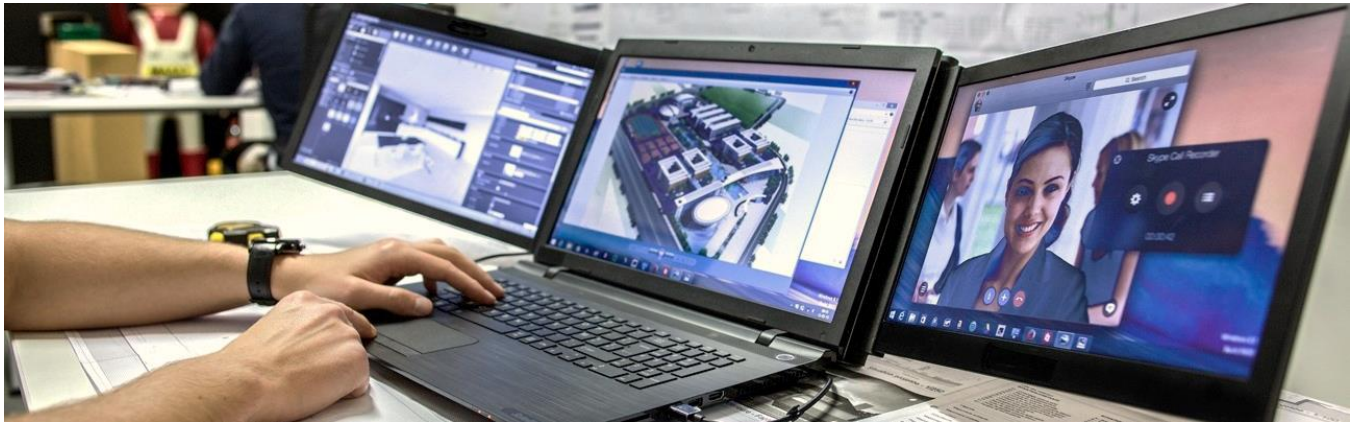
Figure 1: A 3-way display is a reconfigurable form factor of a personal computer that features one central display and two symmetrically expandable lateral sides. In this work, we examine user-defined gesture input for personal 3-way display devices.
