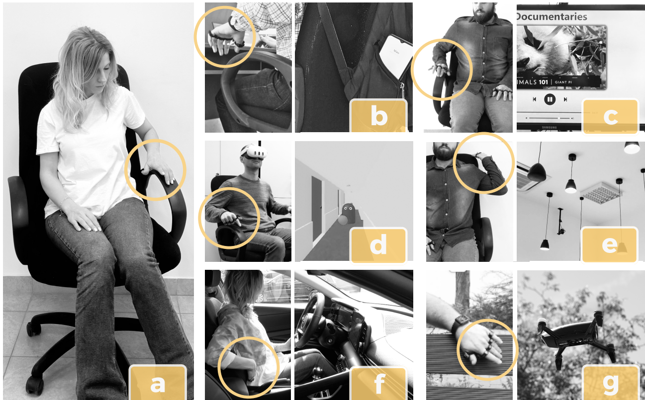
Figure 1: ChairMX is our on-chair gesture input technology for interactive media consumption experiences where chairs are leveraged as input devices, e.g., a tap on the armrest (a) effects a command on a connected device or enables access to digital media on a remote display. We demonstrate applications of ChairMX from smartphone shortcuts (b) to television control (c), interactions in virtual environments (d), control of smart home devices (e), in-vehicle interactions (f), and drone control (g). Due to our system design approach involving a wearable device for the hand, ChairMX is readily deployable to all chairs.
