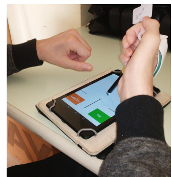
Spinal Cord Injury (C5) Input with a pen attached to the palm with a hand strip
