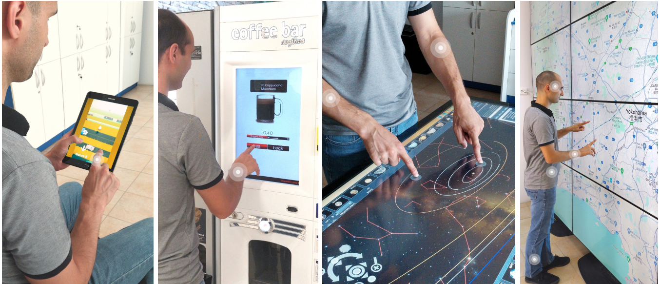
Figure 1: Distal haptics at various body locations—finger, wrist, forearm, or even more distant at whole-body level—provide confirmatory feedback for touch input, especially useful for touchscreens without built-in haptics, like those in these photos. Although consumer wearables—electronic rings, smartwatches, arm bands—can readily deliver distal haptics to connected touchscreens, the novel user experience evoked by spatially decoupling input and output is unknown to interaction designers.
