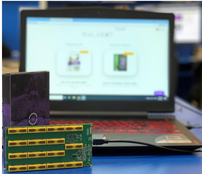
Fig. 2 Walabot device with a 15-antenna array for spatial sensing, distance, and depth measurement; see Figure 3 for examples of gestures collected using this device.
