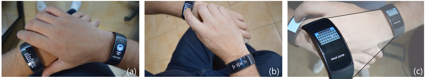
Figure 1. Examples of applications designed for two smartwatches operated in tandem: (a) browsing a list of contacts on one smartwatch, while sending and receiving phone calls on the second watch; (b) visualizing a full-screen detailed view of selected content from one smartwatch on the other; and (c) text entry using a tiny soft keyboard by positioning a cursor on each key with the finger sliding on the touchscreen of the second smartwatch.
